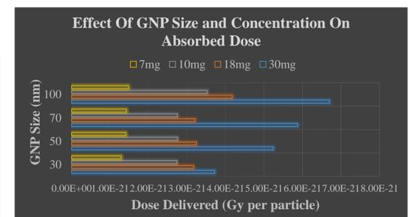
Effect of GNPs size and concentration on absorbed dose (Simulations done with Geant4 code)
